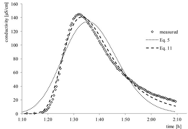
**Fig. 4.** Comparison of measured and simulated conductivity distribution in the test A - Malá Nitra stream, exp. Nr. 12-III (785 m).
