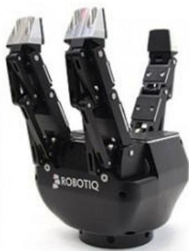
Fig. 1. 3-Finger Adaptive Robotiq® gripper [18].
