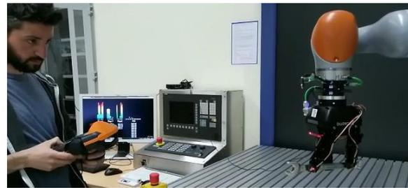
Fig. 9. KUKA LBR iiwa 7 R800 robot grasping a wrench. The pressure values at the fingertip are visualized on the monitor.
