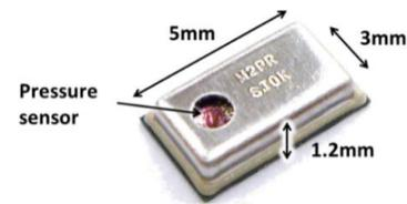
Fig. 2. MPL115A2 sensor from Freescale Semiconductor [17].
