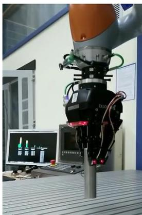
Fig. 8. KUKA LBR iiwa 7 R800 robot grasping a metal cylinder. The pressure values at the fingertip are visualized on the monitor in the background.
