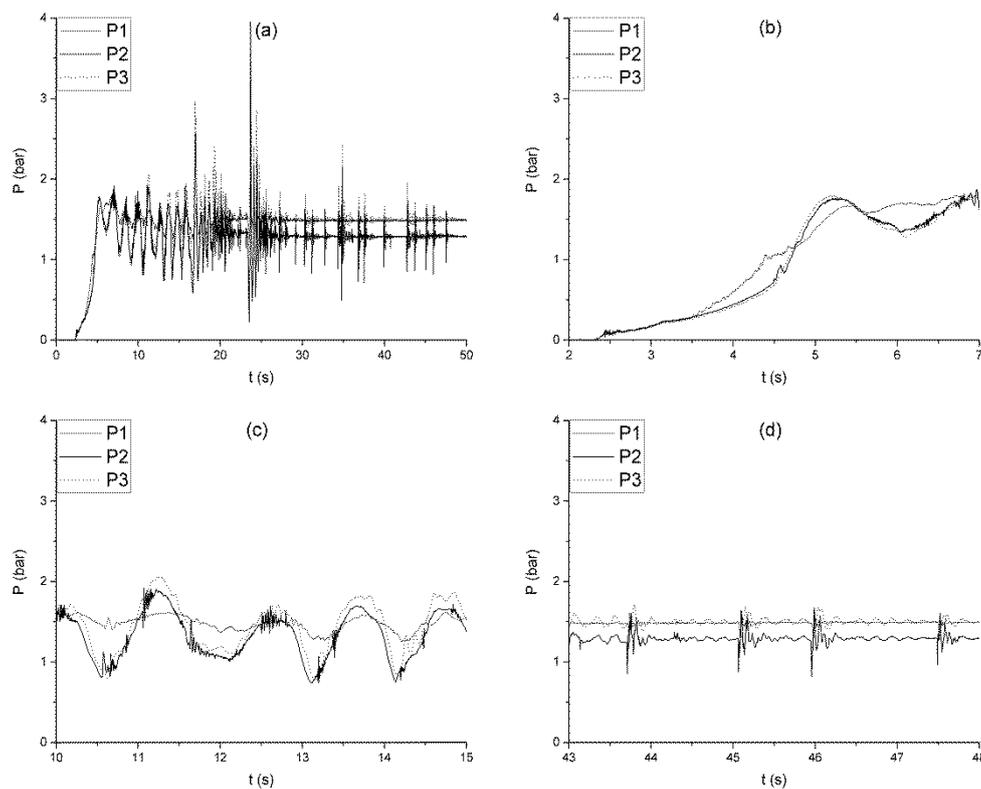
**Figure 3.** Pressure transient for  $\psi_d = 0\%$ ,  $\psi_u = 100\%$ ,  $d = 6.4$  mm (S configuration).
