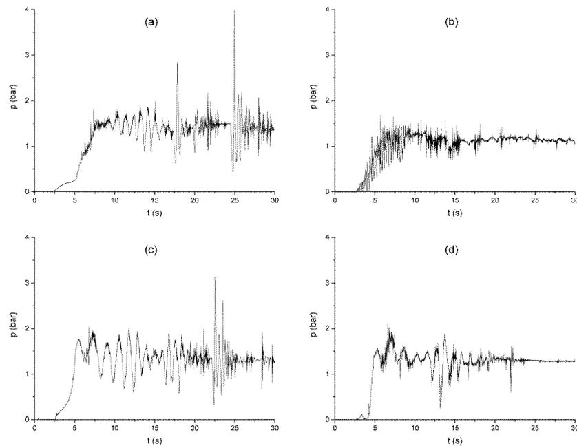
**Figure 5.** Pressure transients for  $\psi_d = 0\%$  with S configuration and: (a)  $\psi_u = 25\%$ ,  $d = 6.4$  mm; (b)  $\psi_u = 25\%$ ,  $d = 25.4$  mm; (c)  $\psi_u = 100\%$ ,  $d = 6.4$  mm; (d)  $\psi_u = 100\%$ ,  $d = 25.4$  mm.
