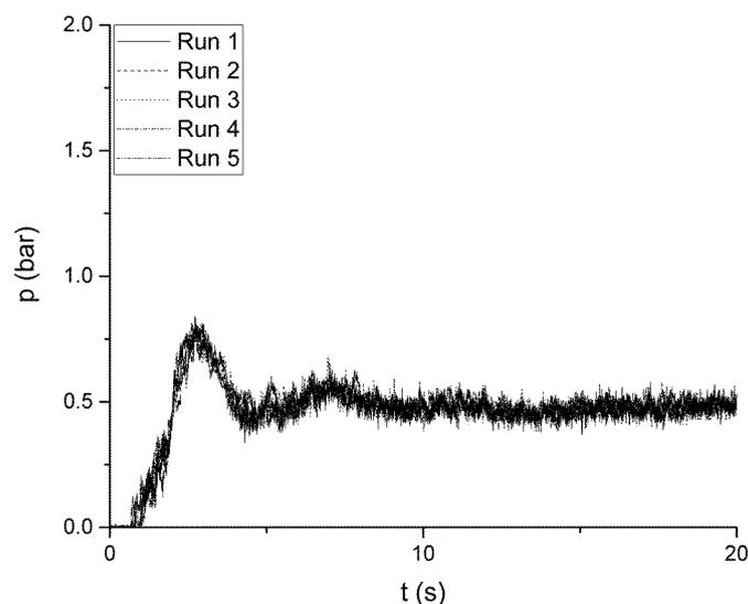
**Figure 2.** Pressure transients for all runs with  $\psi_d = 100\%$ ,  $\psi_u = 50\%$ ,  $d = 6.4$  mm (S configuration).
