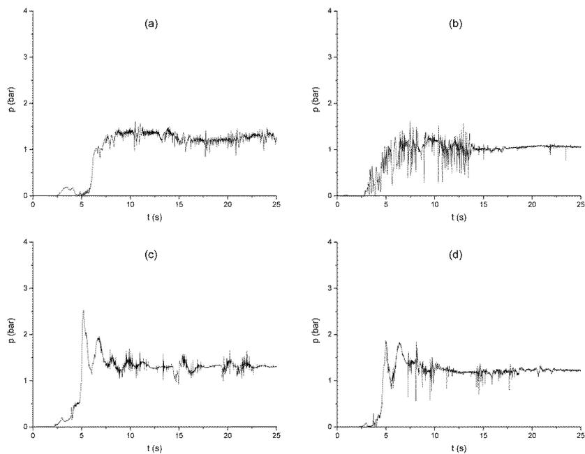
**Figure 6.** Pressure transients for  $\psi_d = 25\%$  with S configuration and: (a)  $\psi_u = 25\%$ ,  $d = 6.4$  mm; (b)  $\psi_u = 25\%$ ,  $d = 25.4$  mm; (c)  $\psi_u = 100\%$ ,  $d = 6.4$  mm; (d)  $\psi_u = 100\%$ ,  $d = 25.4$  mm.
