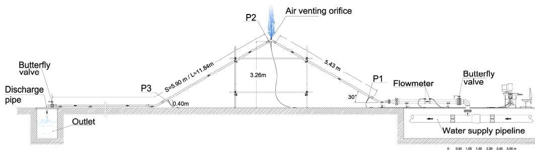
Figure 1. Experimental set-up.
