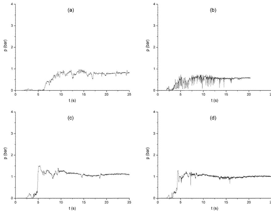
**Figure 7.** Pressure transients for  $\psi_d = 50\%$  with S configuration and: (a)  $\psi_u = 25\%$ ,  $d = 6.4$  mm; (b)  $\psi_u = 25\%$ ,  $d = 25.4$  mm; (c)  $\psi_u = 100\%$ ,  $d = 6.4$  mm; (d)  $\psi_u = 100\%$ ,  $d = 25.4$  mm.
