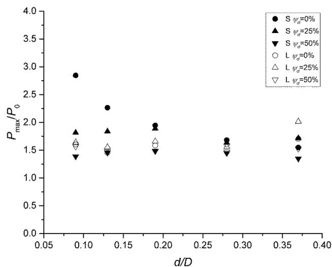
Figure 10. Average pressure surges for S and L configurations at varying  $\psi_d$ ,  $d/D$ .
