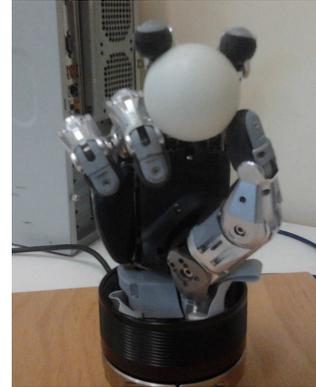
Fig. 1. The Schunk 5 Fingered Hand.
