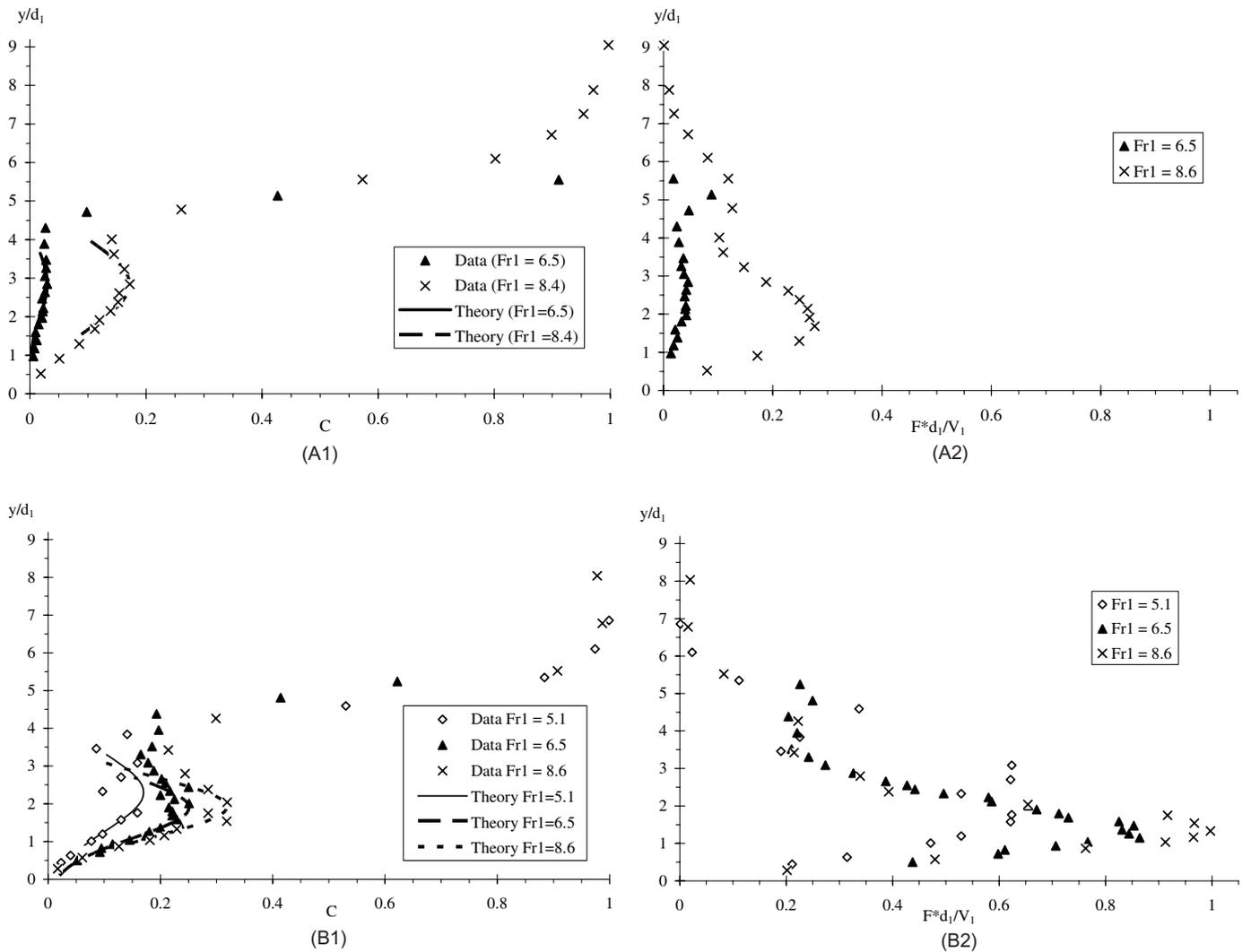
Figure 5 Effects of Reynolds number on dimensionless distributions of void fraction and bubble count rate for three inflow Froude numbers  $Fr_1 = V_1/\sqrt{g * d_1}$ . (A) Small flume data,  $W = 0.25$  m,  $x - x_1 = 0.15$  m. (A1) Void fraction distributions (comparison with Eq. (4)). (A2) Bubble count rate distributions. (B) Large flume data,  $W = 0.5$  m,  $x - x_1 = 0.3$  m. (B1) Void fraction distributions (comparison with Eq. (4)). (B2) Bubble count rate distributions.
