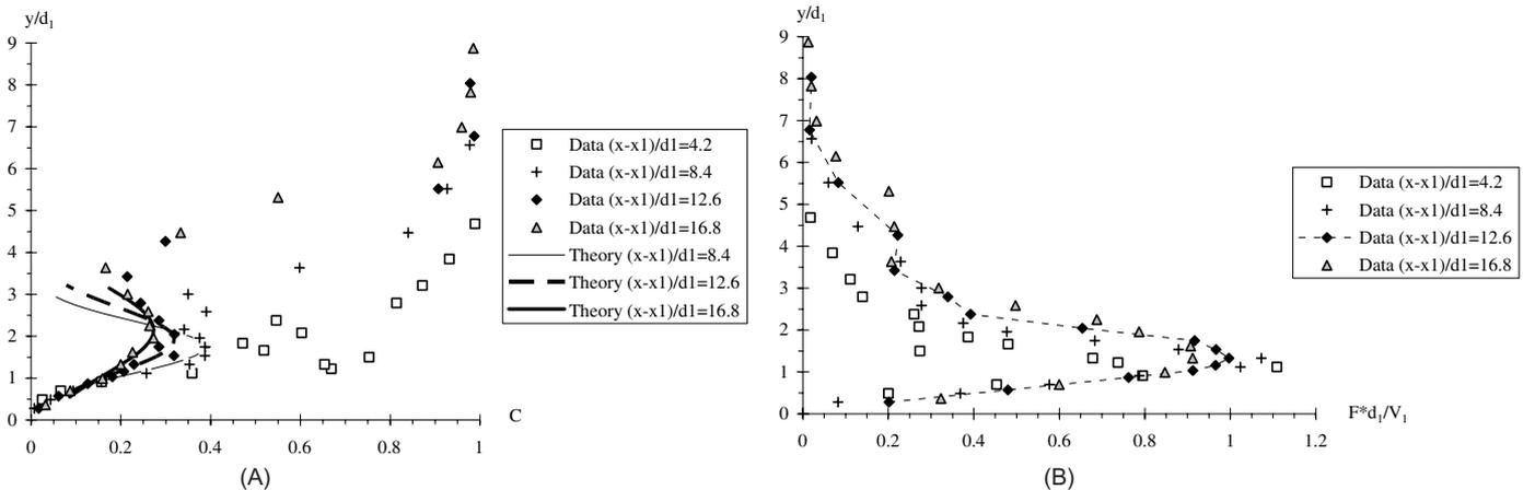
Figure 4 Dimensionless distributions of void fraction and bubble count rate –  $Fr_1 = 8.6$ ,  $Re_1 = 9.8E + 4$ ,  $d_1 = 0.024$  m,  $x_1 = 1.0$  m,  $W = 0.50$  m,  $x - x_1 = 0.1, 0.2, 0.4$  m. (A) Void fraction distributions (comparison with Eq. (4)). (B) Bubble count rate distributions.
