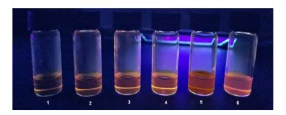
**Figure 2.** The AIE self-assembly naked-eye test as can be appreciated under an UV-visible lamp at 365 nm. Vial 1: 0.1 mM TCE solution of compound L. Vials 2-6 TCE/hexane 0.1 mM solutions in the increasing ratio: 20, 40, 60, 70, 80%.
