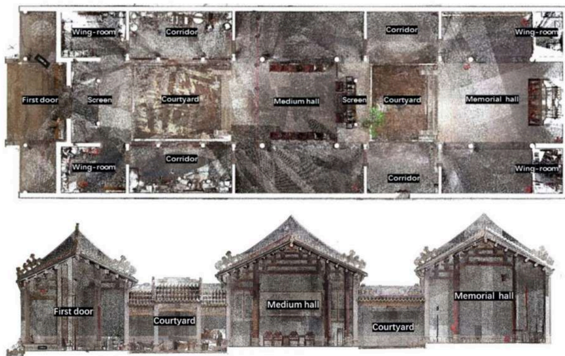
Figure 8. Layout and side view of Wen Ancestral Hall. A top view and a side view the Wen Ancestral Hall are drawn in this figure.
