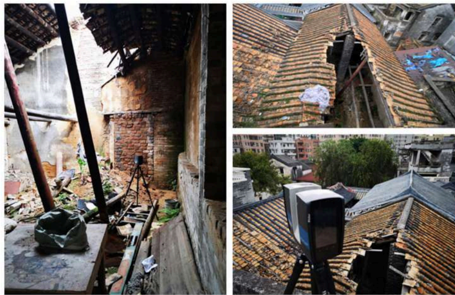
Figure 3. Faro S350 scanner. The Faro scanner is suitable for different kinds of sites, especially for architectural heritage scanning.
