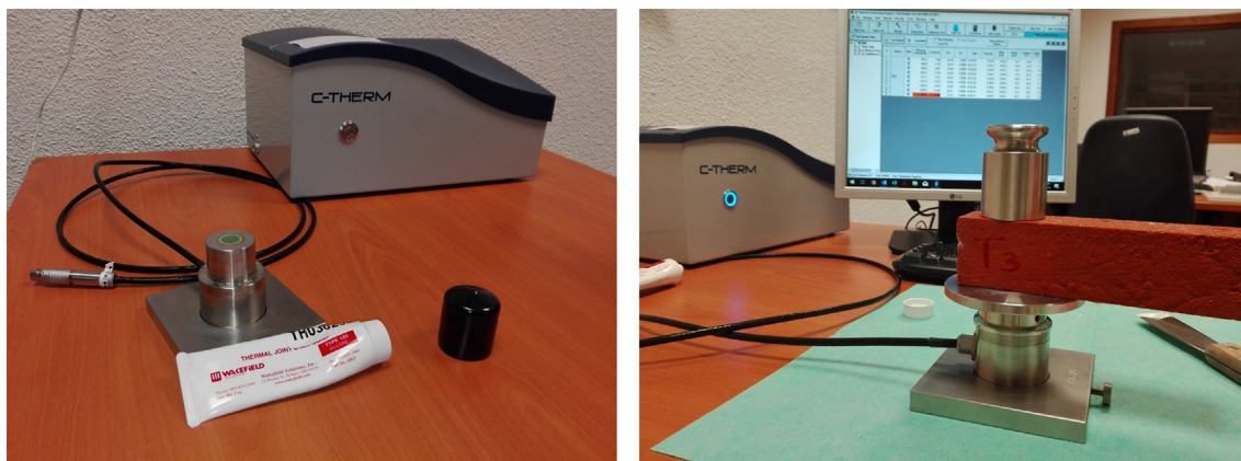
Fig. 4. Equipment used for measuring thermo-physical properties.
