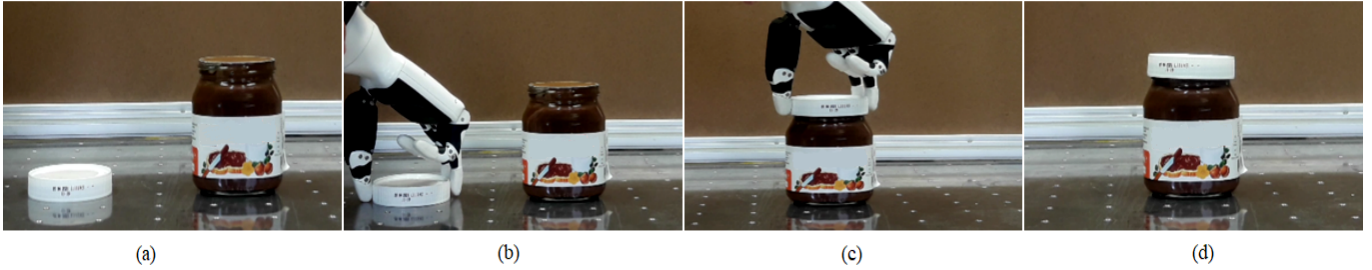
Fig. 12: A robot hand closing a jar, (a) illustrates the jar and its lid, (b) demonstrate the robot hand grasping the lid in a tripod (3 fingered) precision grasp, (c) shows the scenario where the lid is placed on the jar while maintaining a stable grasp, (d) displays the final pose of jar with the lid being screwed onto it.
