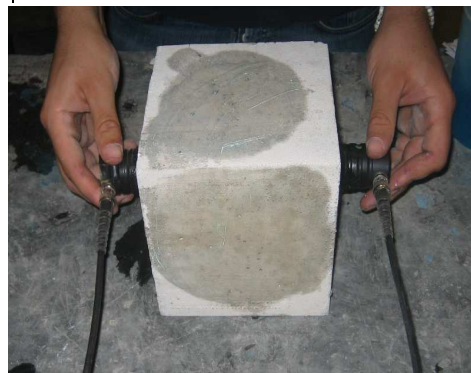
Fig.6 - Application of ultrasonic probes
