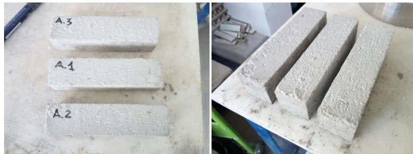
Fig. 1-2 —samples of mortar packaged in number of three for each typologies, for samples A and B
