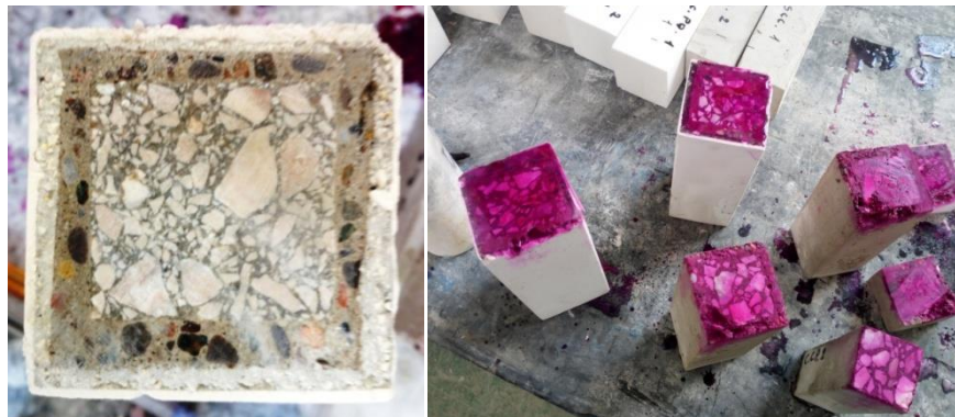
Fig. 3-4 —sample that has just been broken, and just after the phenolphthalein spray
