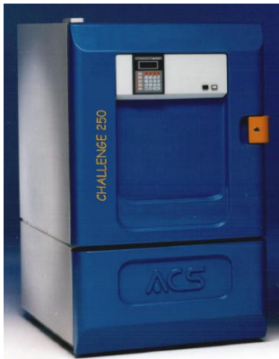
Fig. 9-10 -The climatic chamber for accelerated ageing tests and the diagram showing the testing program, which represents the climate of the city of Naples
