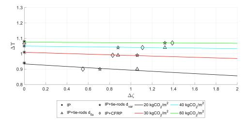
**Figure 7.** Environmental iso-cost curves—absolute performance indicators  $\Delta Y$  (*thermal*)  $-\Delta \zeta$  (*seismic*) for different integrated retrofit solutions and consequent fitting curves as function of the environmental impact.
