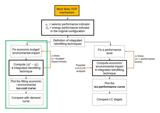
**Figure 1.** Schematics of the proposed procedure for the selection of optimal integrated retrofitting techniques for OOP failure modes in masonry buildings. Only the part framed in green is developed in this paper.
