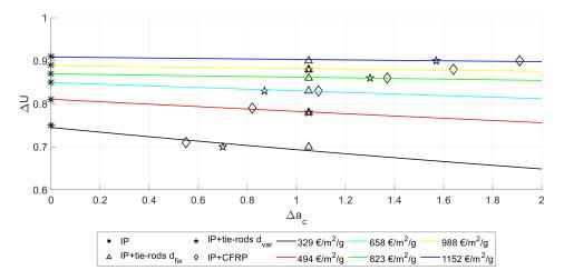
**Figure 4.** Economic iso-cost curves—relative performance indicators  $\Delta U$  (*thermal*)  $-\Delta a_c$  (*seismic*) for different integrated retrofit solutions and consequent fitting curves as function of the economic budget.
