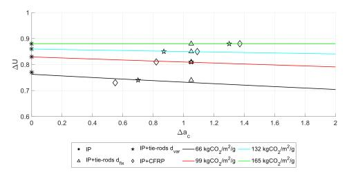
**Figure 5.** Environmental iso-cost curves—relative performance indicators  $\Delta U$  (*thermal*)  $-\Delta a_c$  (*seismic*) for different integrated retrofit solutions and consequent fitting curves as function of the environmental impact.
