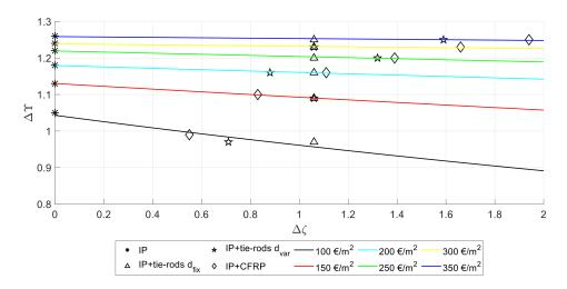
**Figure 6.** Economic iso-cost curves—absolute performance indicators  $\Delta Y$  (*thermal*)  $-\Delta \zeta$  (*seismic*) for different integrated retrofit solutions and consequent fitting curves as function of the economic budget.
