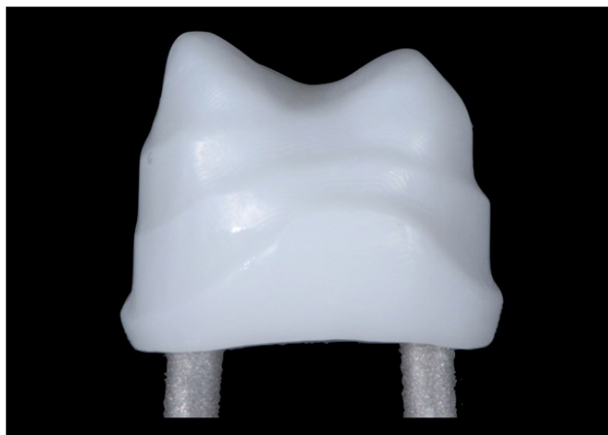
Fig. 3. Sample of Group 3: anatomically-guided, designed to keep constant the thickness of the overlying porcelain veneering (AG).
