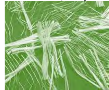
Fig. 107 Macrofibre, microfibre e fibre fibrillate in polipropilene / Macrofibres, microfibrils and fibrillated fibers in polypropylene
