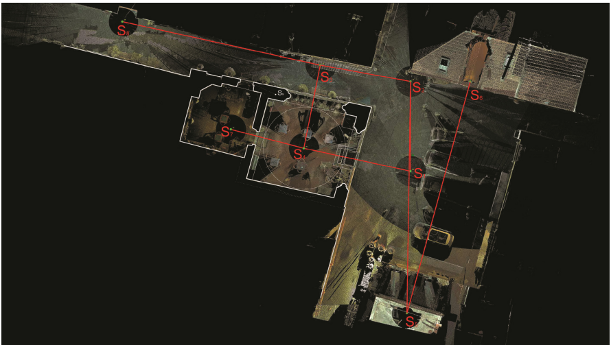
Fig. 1. Sedile Dominova geometric survey, the plan with the 3D scans positioned.
