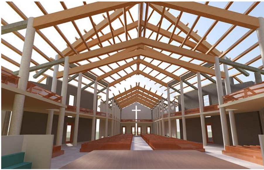
Figure 9. Render of the laminated wood covering during assembly
