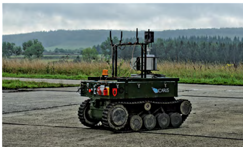
Figure 13. RMA tEODor UGV with the 3D mapping hardware.
