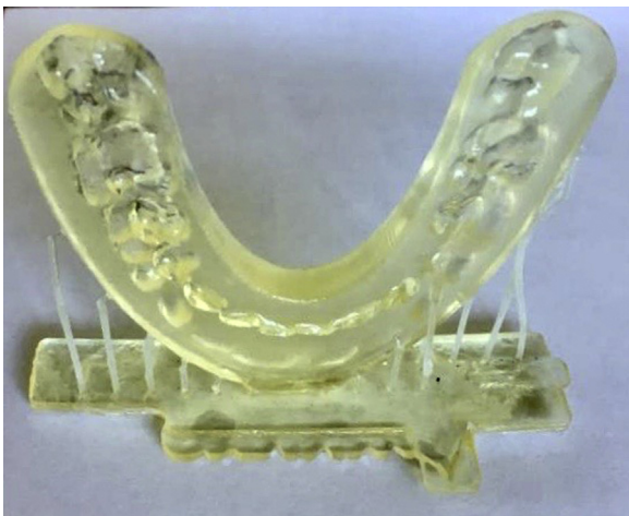
Fig. 2. Three-dimensional printed surgical splint.
