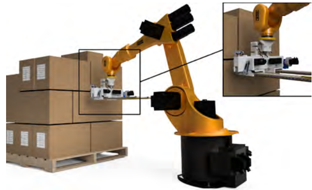
Fig. 1. Rendering of the gripper prototype attached to an industrial robot.
