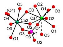
**Figure 3.** Coordination environments around the Ca1 and Ca2 sites in hydroxyapatite. Dashed lines: Ca-O interactions >2.8 Å.
