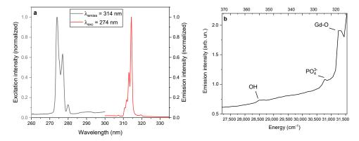
**Figure 8.** (a) HA-Gd excitation (detecting the emission at 314 nm) and emission (excitation at 274 nm) spectra; (b) vibronic bands and assignments in the HA-Gd emission spectrum.
