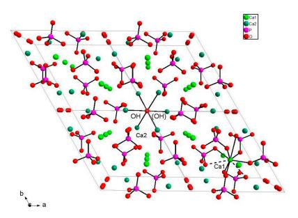
**Figure 4.** Three-dimensional framework of HA-Eu4 sample, showing details of Ca1O<sub>6</sub> metaprisms, and Ca2<sub>6</sub>(OH)<sub>2</sub> groups. The OH groups correspond to O4 atoms. Ca1-O3 bonds are dashed for clarity.
