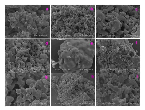
**Figure 1.** Scanning electron microscopy (SEM) images of Eu- and Gd–doped HA samples synthesized here. Detail of: HA-Eu1 at 5  $\mu$ m (**a**) and 10  $\mu$ m (**b**); HA-Eu2 at 5  $\mu$ m (**c**) and 10  $\mu$ m (**d**); HA-Eu3 at 5  $\mu$ m (**e**) and 10  $\mu$ m (**f**); HA-Eu4 at 5  $\mu$ m (**g**) and 10  $\mu$ m (**h**); HA-Gd at 5  $\mu$ m (**i**).
