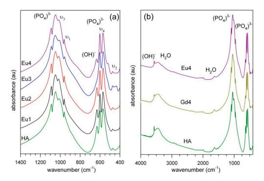
**Figure 5.** (a) Fourier transform infrared (FTIR) spectra of Eu-doped HA samples in comparison with undoped HA in the low-frequency ( $<1200 \text{ cm}^{-1}$ ) lattice mode region; (b) comparison between the spectra of samples HA-Gd and HA-Eu4 in the full range 4000–400 cm<sup>-1</sup>.
