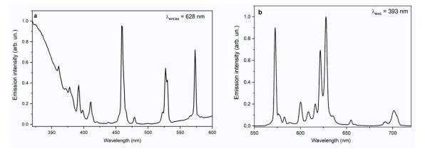
**Figure 6.** (a) Normalized excitation spectrum of HA-Eu4, detecting the emission at 628 nm. (b) Emission spectrum of HA-Eu4, collected upon excitation at 393 nm.
