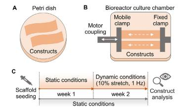
**Figure 2.** Static versus dynamic culture experimental plan. (A) Constructs in static conditions. (B) Constructs in dynamic conditions, grasped between the two opposite clamps. (C) Timeline of the performed culture protocols.
