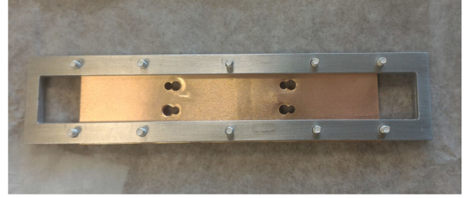
FIG. 3. Top view of the longitudinal copper slab surrounded by the aluminum frame used during the NEG deposition. The four holes are for the correct alignment of the coated slab in the DUT during THz measurements.
