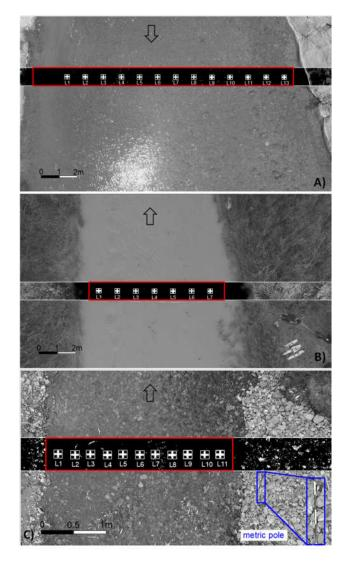
**Figure 3.** Frames acquired at (**A**) Noce, (**B**) Bradano, and (**C**) Basento Rivers. Dark zones represent frames after contrast stretching, enhancing the contrast between tracers and background. Regions of interest (ROIs) are shown in red squares and locations of reference velocity measurements as white crosses. The main flow direction is indicated by arrows. A zoom-in of the metric pole is shown in (C).
