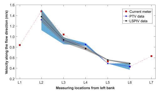
**Figure 9.** Comparison between surface velocity estimations computed with PTV and LSPIV for experiments conducted in the Bradano River. Shaded regions indicate standard deviations between frame sequences. Values recorded with the current meter are indicated by red squares.
