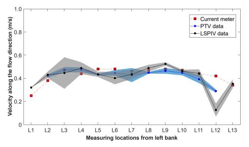
**Figure 7.** Comparison between surface velocity estimation computed with PTV (blue line) and LSPIV (black line) for experiments carried out in the Noce River at different frame windows. Shaded regions indicate standard deviations between frame sequences. Values recorded with the current meter are indicated by red squares.
