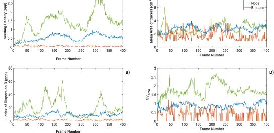
Figure 5. Comprehensive overview of seeding behaviour during considered acquisition time for each study case. (A) Seeding density in particles per pixel (ppp), (B) mean area of tracers in  $\text{cm}^2$ , (C) dimensionless dispersion index, and (D) coefficient of variation of the tracers' area.
