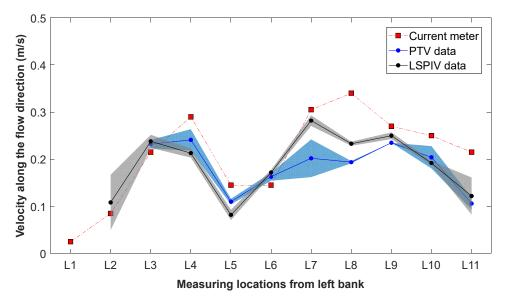
**Figure 11.** Comparison between surface velocity estimations computed with PTV and LSPIV for experiments conducted on frame windows in the Basento River. Shaded regions indicate standard deviations between frame sequences. Values recorded with the current meter are also reported.
