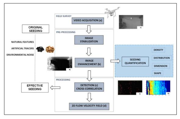
**Figure 2.** Workflow of surface flow estimation, including seeding quantification and optical methods: (**A**) video acquisition; (**B**) image enhancement; (**C**) feature detection; (**D**) 2D flow velocity field.
