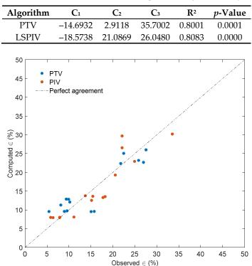
Figure 12. Error predicted by multiple regression analysis vs. error observed with PTV and LSPIV.
