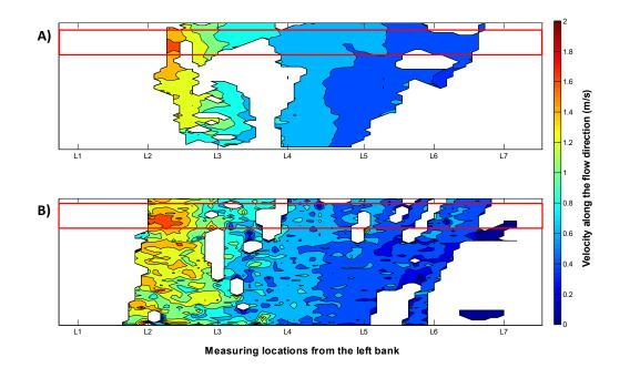
**Figure 8.** Examples of flow velocity maps calculated with (**A**) PTV and (**B**) LSPIV techniques for frame window FW5 on Bradano River. Red squares represent ROI considered for the analysis.
