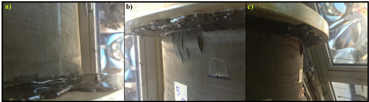
14 15 16 17 18 19 20 21 22 23 24 25 26 27 Fig. 8. Highlights from compression tests on CFRP skirts showing the specific damaging mechanisms due to 28 compression load 29
