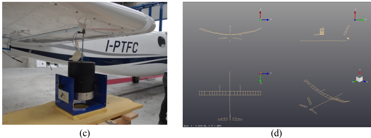
Fig. 1 – GVT on a Small Commuter Airplane (a); measuring points (b); electrodynamic shaker excitation (c) and example of mode-shape (d)
