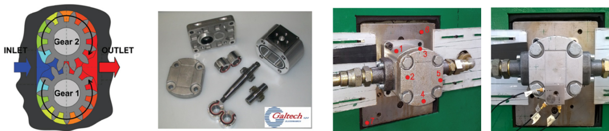
Figure 2. External gear pump (left) and accelerometer positions for test measurements (right).
