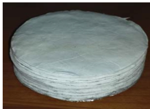
Fig. 8 – Specimens for the impedance tube
