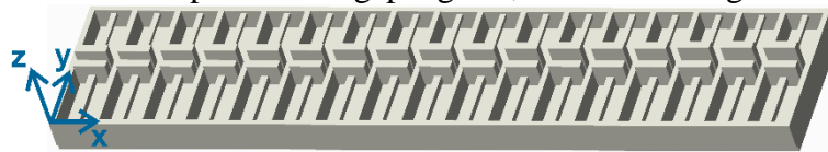
Figure 1: Schematic representations of the metamaterial beam with non-symmetric resonators at each unit cell [7].
