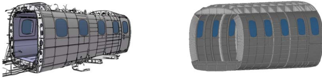
Figure 3 (a) Fuselage CAD model; (b) Fuselage FEM model
