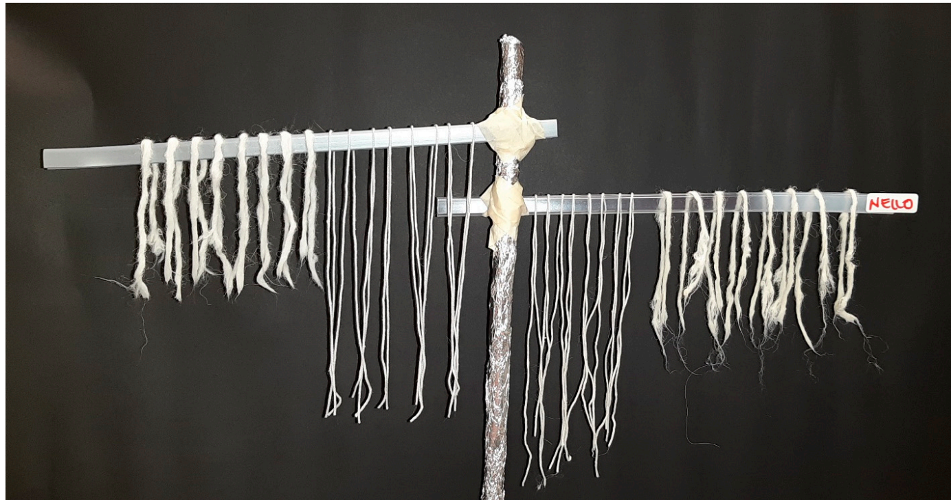
Figure 2. Image of the post-etching cotton and wool fibers: the treatment with aluminum potassium sulfatate ( left ) and lemon juice ( right ).
