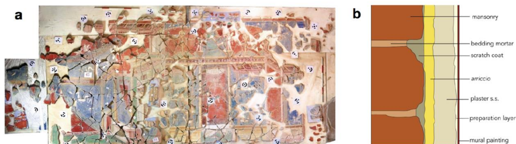
Fig. 4. (a) Recomposition of fragments belonging to the west wall (photos by G. Di Maio, Geomed archives); image width ca. 2 m. The samples of this study come from this part of the triclinium; (b) sketch section of a typical Roman plaster, inferred from the Vitruvius' treatise, redrawn after [39].
