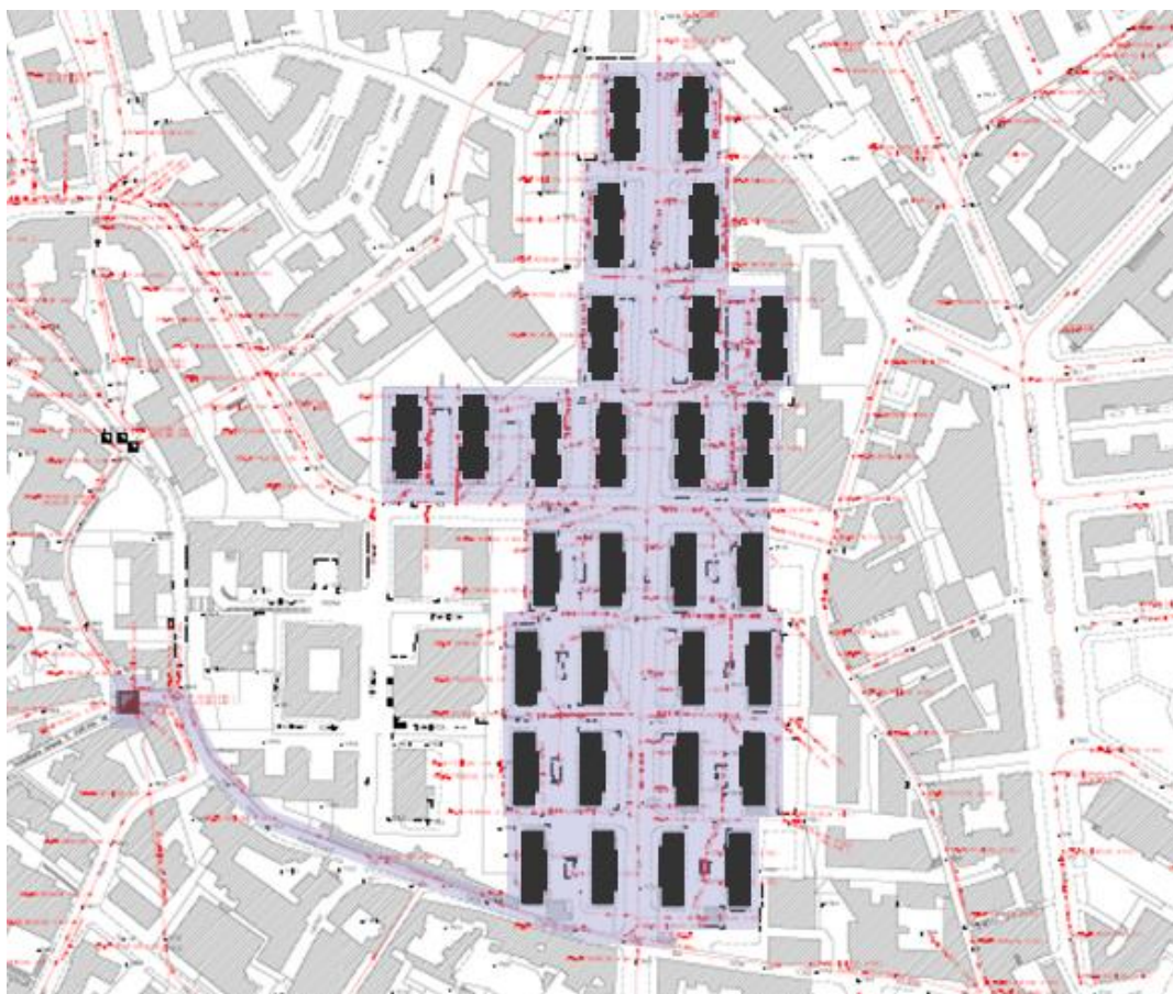
Fig. 9 Plan of the Rione Gemito sewage network
