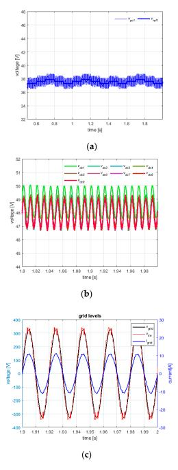
**Figure 11.** (a) PV voltage and MPPT voltage reference of power cell#1, (b) DC-link voltages, (c) PVGs irradiance of  $1000 \text{ W/m}^2$  for the 1st power cell and of  $554 \text{ W/m}^2$  for the remaining eight cells: steady-state behavior of grid current (blue line), modulated voltage (red line), and the grid voltage (black line), in an observation window of (1.9 s, 2 s).
