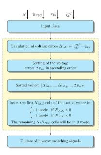
Figure 4. Sorting algorithm flow-chart.
