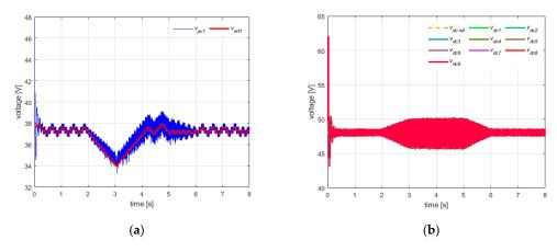
Figure 16. (a) PV voltage and MPPT voltage reference of power cell#1, (b) DC-link voltages.
