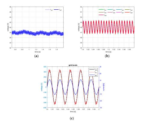
**Figure 8.** (a) PV voltage and MPPT voltage reference of power cell#1, (b) DC-link voltages, (c) PVGs irradiance of 603.31 W/m<sup>2</sup>: steady-state behavior of grid current (blue line), modulated voltage (red line), and the grid voltage (black line), in an observation window of (1.9 s, 2 s).
