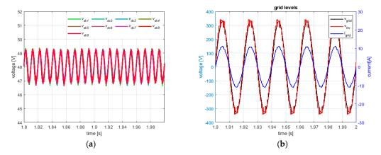
**Figure 7.** (a) DC-link voltages, (b) PVGs (Photovoltaic Generators) irradiance of 1000 W/m<sup>2</sup>: steady-state behavior of grid current (blue line), modulated voltage (red line), and the grid voltage (black line), in an observation window of (1.9 s, 2 s).
