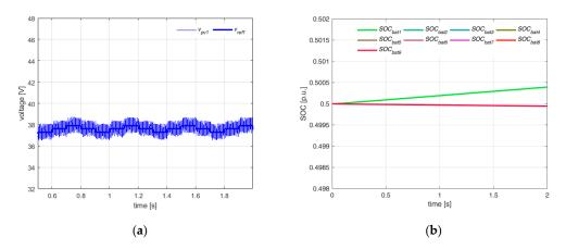
**Figure 9.** (a) PV voltage and MPPT voltage reference of power cell#1, (b) SOC vs time of the nine power cell (green line, cell#1, red line, the remaining 8 cells).
