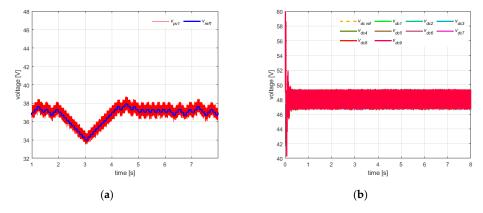
Figure 14. (a) PV voltage and MPPT voltage reference of power cell#1, (b) DC-link voltages.
