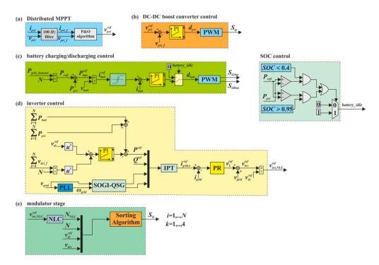
**Figure 3.** Control section: (**a**) Distributed MPPT, (**b**) boost converter control, (**c**) bidirectional dc-dc and SOC (State of Charge) control, (**d**) inverter control, (**e**) modulator stage with sorting algorithm.
