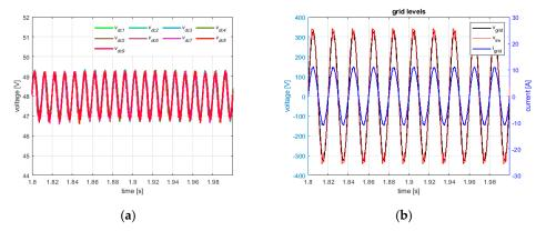
**Figure 18.** (a) DC-link voltages, (b) PVGs irradiance of 1000 W/m<sup>2</sup> for the 1st power cell and of 554 W/m<sup>2</sup> for the remaining eight cells: steady-state behavior of grid current (blue line), modulated voltage (red line), and the grid voltage (black line), in an observation window of [1.8 s, 2 s].
