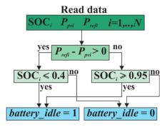
Figure 5. SOC control flowchart.
