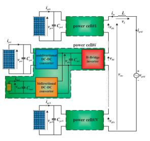
**Figure 1.** The architecture of 2N + 1-level grid-tied photovoltaic (PV).
