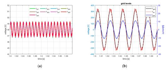
**Figure 10.** (a) DC-link voltages, (b) PVGs irradiance of  $1000 \text{ W/m}^2$  for the 1st power cell and of 554 W/m<sup>2</sup> for the remaining eight cells: steady-state behavior of grid current (blue line), modulated voltage (red line), and the grid voltage (black line), in an observation window of (1.9 s, 2 s).
