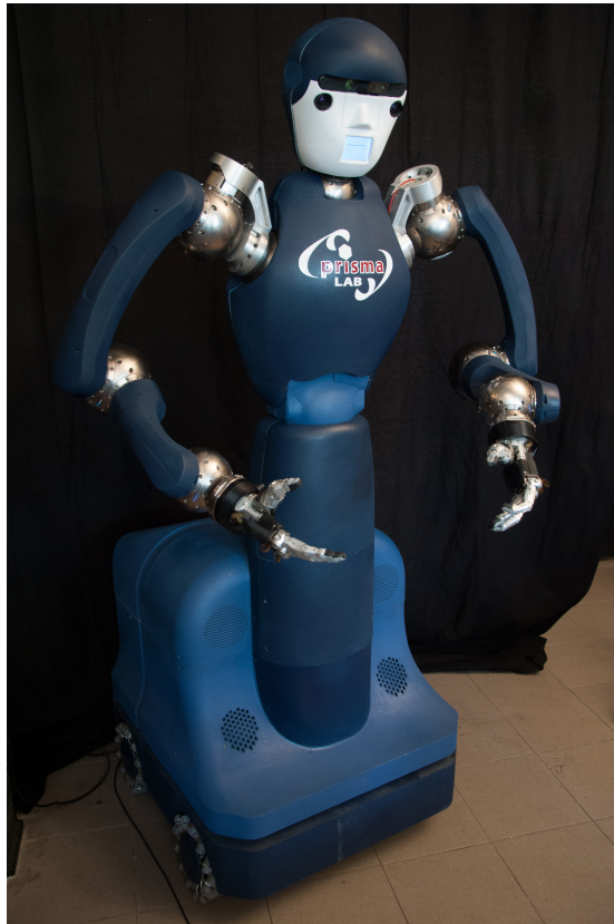
Fig. 1. The RoDyMan robotic platform equipped with two Schunk SVH hands as end-effectors.
