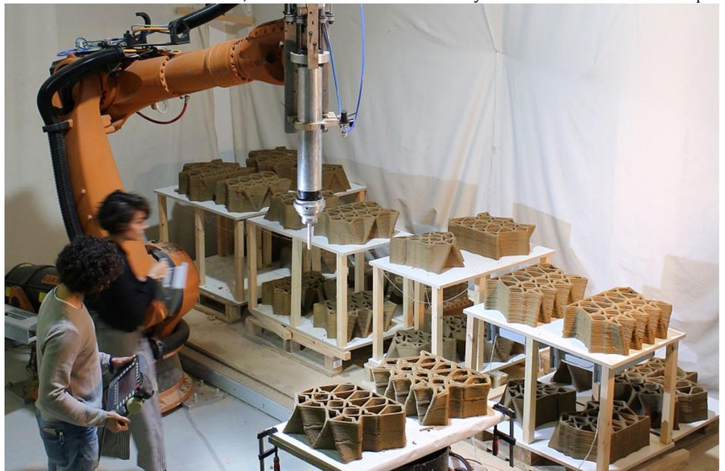
Fig.1- 3D printing phase of TerraPerforma Project of the IAAC (Institute of Advanced Architecture Catalonia). @iaac.net.
