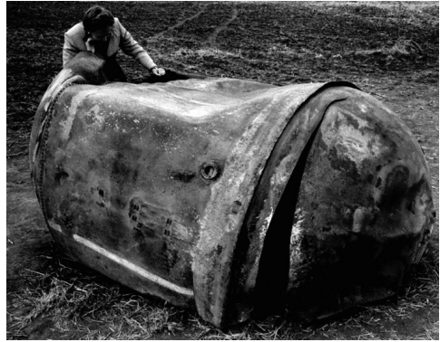
Fig. 16 - Orbital debris. Recovered object. Main tank of a Delta 2 launch vehicle which landed in Texas, on 22.01.1997. http://orbitaldebris.jsc.nasa.gov/reentry/recovered.html
