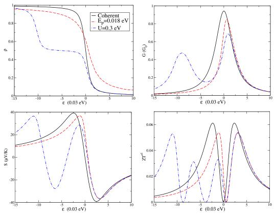
**Figure 2.** Level density  $\rho$  (**Top Left**); charge conductance G (in units of the conductance quantum  $G_0$ ) (**Top Right**); Seebeck coefficient S (in units of  $\mu V/K$ ) (**Bottom Left**); and electronic thermoelectric figure of merit  $ZT^{el}$  (**Bottom Right**) as a function of level energy  $\epsilon$  (in units of 0.030 eV) at the temperature T = 100 K.
