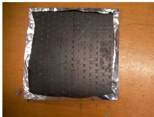
Figure 22. Photographs of the residue of the nanofilled panel after the cone calorimeter test performed at irradiance 35 \text{ kW/m}^2 .
