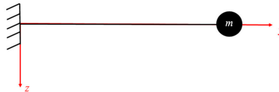
Figure 2. Mono-dimensional scheme of the support with the local coordinate system and the mass corresponding to half the rotor mass concentrated at the free end.
