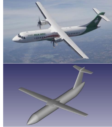
Fig. 5. Comparison between the ATR72 (above) and the JPAD parametric CAD model (below).
