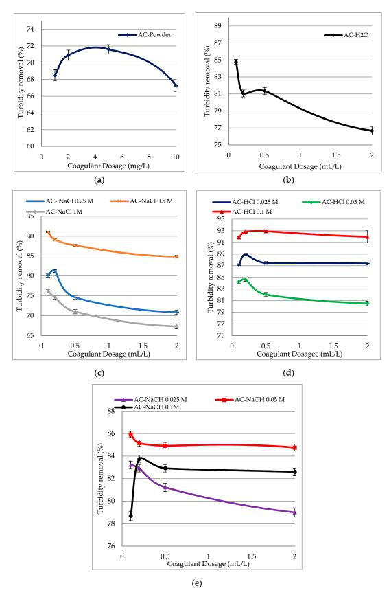
**Figure 3.** Effect of dosage on turbidity removal efficiency for coagulants extracted with different solvents: (a) AC powder; (b) AC extracted by distilled water; (c) AC extracted by NaCl solution; (d) AC extracted by HCl solution; (e) AC extracted by NaOH solution.
