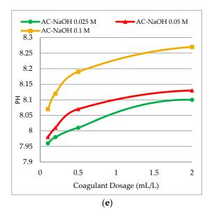
**Figure 4.** Effect of coagulant dosage on pH: (a) AC powder; (b) AC extracted by distilled water; (c) AC extracted by NaCl solution; (d) AC extracted by HCl solution; (e) AC extracted by NaOH solution.
