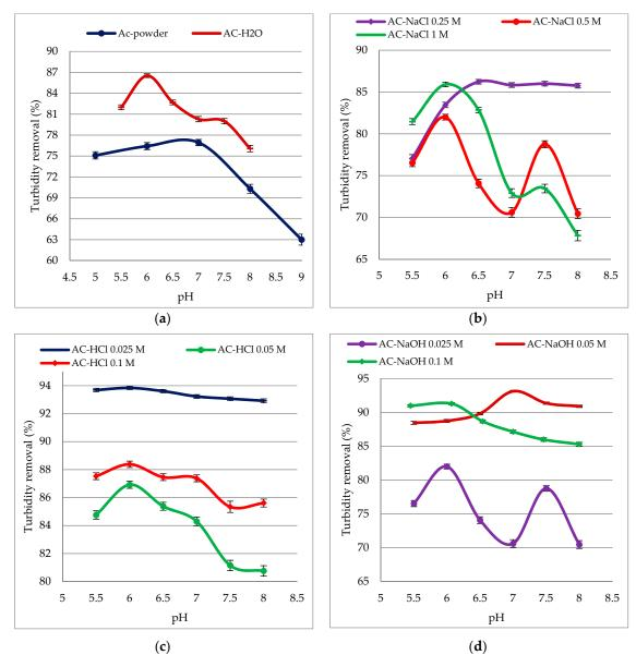
**Figure 5.** Effect of pH on turbidity removal efficiency for different coagulants at their optimal dosage: (a) AC extracted by distilled water; (b) AC extracted by NaCl solution; (c) AC extracted by HCl solution; (d) AC extracted by NaOH solution.
