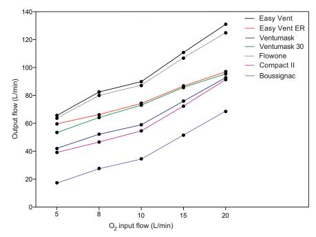
Fig. 1. Output flow generated by each device according the  $O_2$  input flow.
