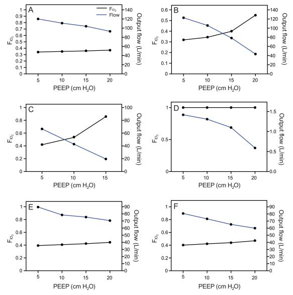
Fig. 2. Static test for each device performed with 4 levels of PEEP (5, 10, 15, and 20 cm H<sub>2</sub>O) with oxygen source flows of 20 L/min. (A) Easy Vent. (B) Flowone. (C) Compact II. (D) Boussignac. (E) Ventumask 30. (F) Ventumask.
