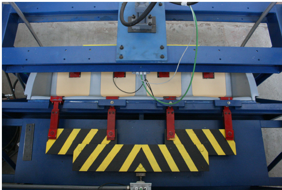
Fig.2 Loads distribution system.
