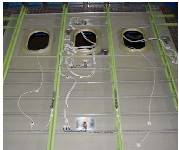
Figure 2 Strain gage and rosette configuration on side A.
