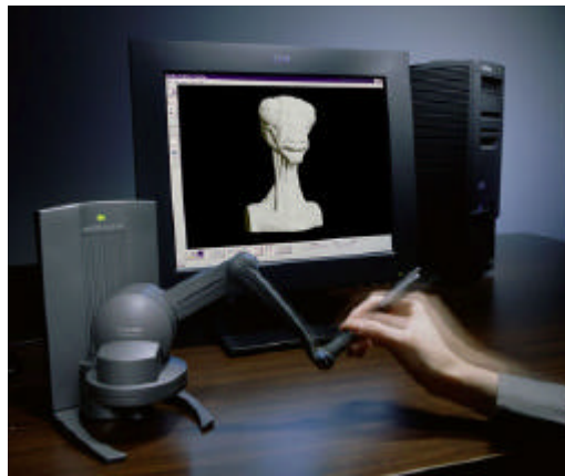
Fig. 4.18. - SensAble Technologies force feedback system.
