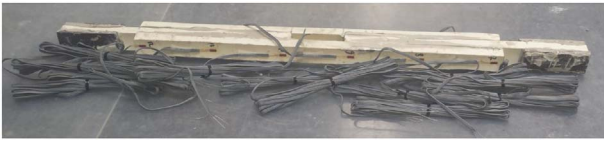
Fig. 7. Joint sample “I” (after strain gauges application).
