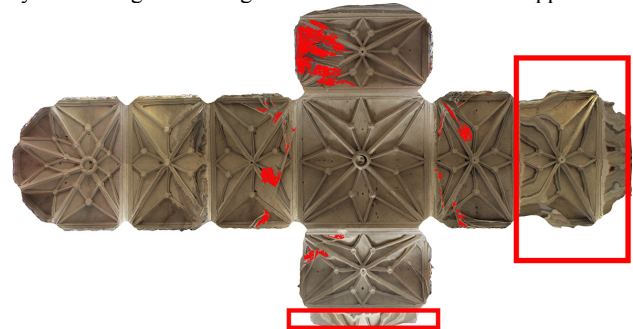
Figure 10 Paris. St. Gervais et St Protais rib vault system. Plan view by 3D textured model from Agisoft PhotoScan.
