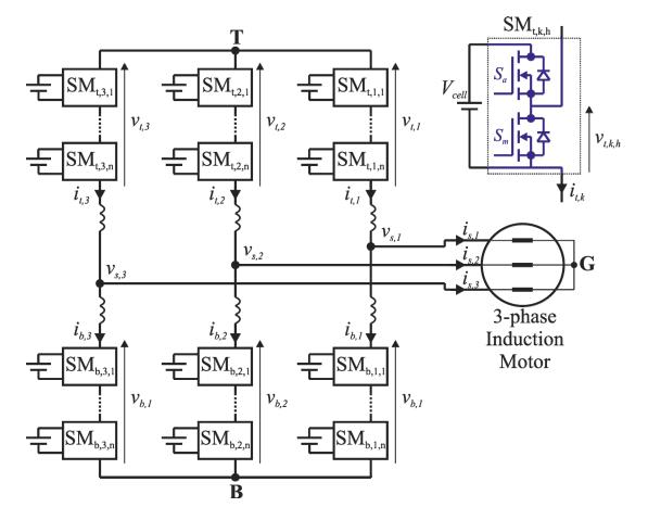
Figure 1. Modular multilevel converters (MMC) power topology.
