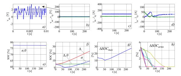
Figure 5. Numerical results for zero speed: (a) zoom of x motor voltage component; (b) x,y motor voltage components; (c) x,y motor current components; (d) x,y circulating current components; (e) half of the zero-sequence component of the arms sum SOCs; (f) unbalance SOC terms; (g) difference between the maximum and the minimum SOC of all cells; and, (h) difference between the maximum and the minimum SOC of the six arms.
