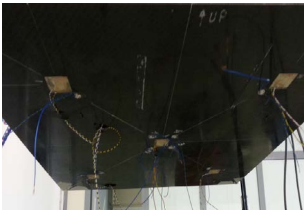
Fig. 1: Piezoceramic patches bonded on the panel
