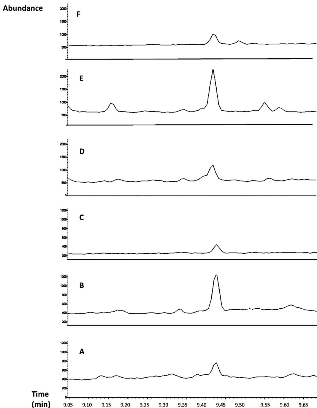
**Figure 3.** Representative GC traces of the monitored ions. The graphic corresponds to the sample goat/Decollatura/June 2014 in Table 1. Panels A, B, and C refer to the monitoring of ions at  $m/z$  187, 201, and 280. Panels D, E, and F refer to the corresponding deuterated ions at  $m/z$  189, 205, and 284. The retention time of the analyte is 9.42 min.
