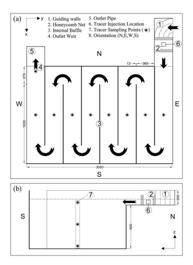
**Figure 2.** Schematic plan view of the solute transport case study: (**a**) a contact tank that features meandering flow as indicated by vectors; (**b**) cross-sectional view of the channel inlet and Compartment 1 (dimensions in mm).
