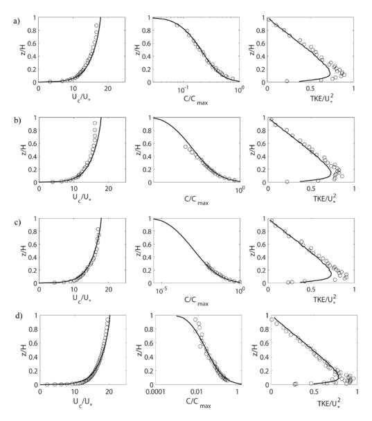
**Figure 5.** Comparison of numerical results of carrier velocity, sediment concentration and total kinetic energy (TKE) for tests by [93]: (a) PS03; (b) PS08; (c) PS13; and a test by [48]: (d) NS1. Adapted from [43]. The circles represent the experimental data, and the solid line represents the numerical result.
