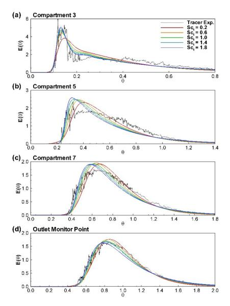
**Figure 3.** Residence time distribution curves predicted for different sampling points at the tracer sampling points at: (a)  $z/H_t = 0.5$  in Compartment 3; (b)  $z/H_t = 0.5$  in Compartment 5; (c)  $z/H_t = 0.5$  in Compartment 7; and (d) at the outlet.
