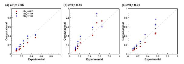
**Figure 4.** Dispersion index values predicted numerically and experimentally for the contact tank tracer sampling points at (**a**)  $z/H_t = 0.05$  in; (**b**)  $z/H_t = 0.5$ ; (**c**)  $z/H_t = 0.95$ .
