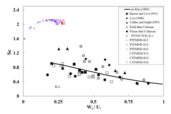
**Figure 6.** Comparison of numerical results (open symbols) with experiments (filled symbols) contributed by different authors for  $Sc_t$  in a particle-laden, open-channel flow. Adapted from [45] and modified for the present contribution. PTFM/CTFM and PTFMND/CTFMND are dilute and non-dilute models, respectively. S13, S14 and S16 refer to the test cases of [96]. The solid line indicates values obtained from the van Rijn (1984) formula.
