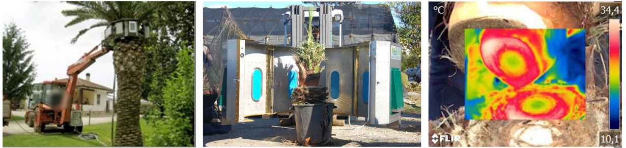
Figure 5. The ring applicator; (a) Ecopalm Ring patented by BIELLE surrounding the palm in closed position (by courtesy of BIELLE srl); (b) cut palm during just after treatment, the applicator is in the open position; (c) thermogram acquisition.
