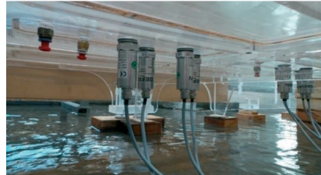
Figure 5. Pressure taps with transducers under the basin floor.
