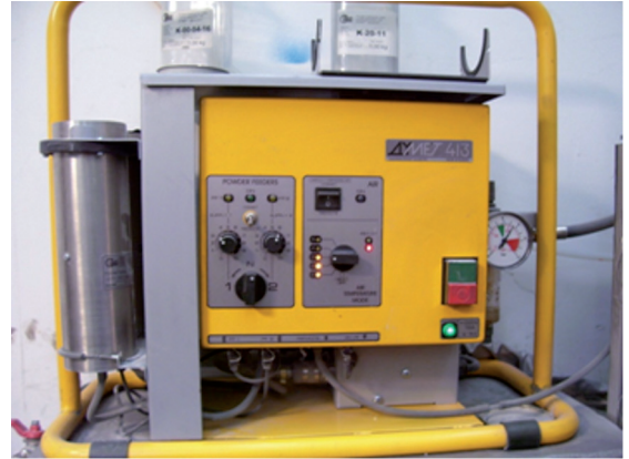
Figure 5: Low pressure Dymet equipment used for the spraying process.
