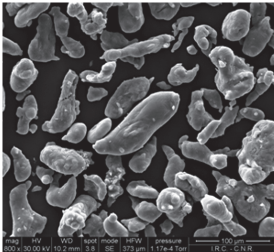
Figure 4: SEM micrograph of the powders used for the cold spray repairing.
