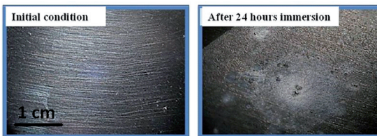
Figure 11: Macrograph of the top surface of the cold spray repair before and after the immersion test.
